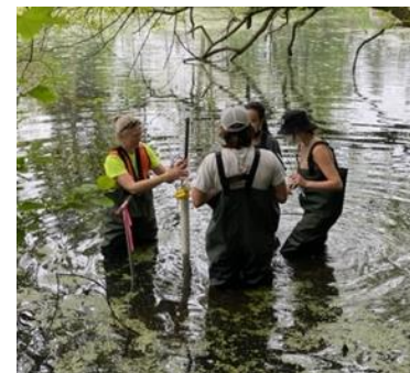
Students from South Hadley High School install water level and pH loggers in Titus Pond with the help of Fuss & O’Neill staff, May 2022
